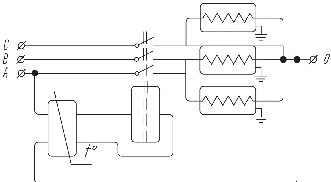
Scheme 3. Connection diagram through thermostat and power contactor
