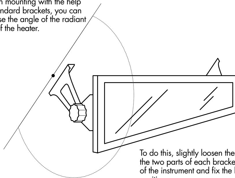
To do this, slightly loosen the thumb bolts connecting the two parts of each bracket. Set the required angle of the instrument and fix the brackets in the selected position.
